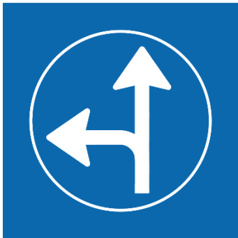
D06-L Mandate to follow one of the driving directions indicated on the board (left, straight ahead)
