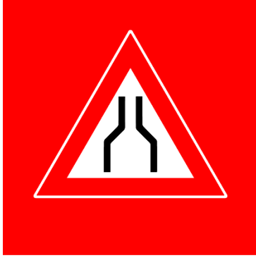
J17 Warning for lane narrowing
