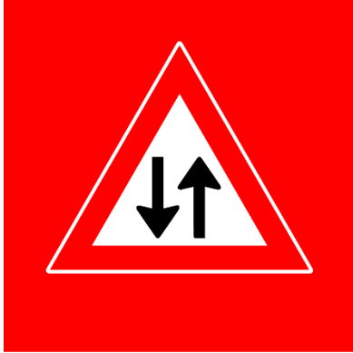
J29 Warning for oncoming traffic
