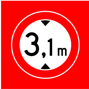
C19 Closed for vehicles and combinations of vehicles, that including load, are higher than the sign states (3,1m)
