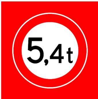
C21 Closed voor vehicles and combinations of vehicles with a total mass higer than the sign states (5,4t)
