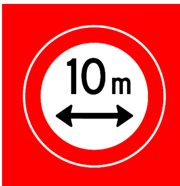
C17 Closed for vehicles and combinations of vehicles, that including load, are longer than the sign states (10M)
