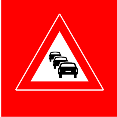
J33 Warning for traffic jam
