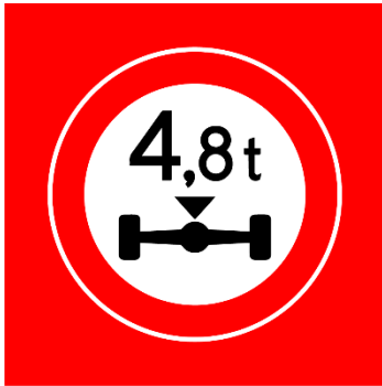
C20 Closed voor vehicles with an axel load higer than the sign states (4,8t)
